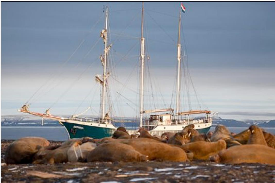
The SV *Antigua* was built in 1957 in Thorne (UK) and served for many years as a fishing vessels, until it was completely re-built in the early 1990s in the Netherlands as a barkentine and equipped as a passenger ship. A barkentine has three masts with square sails on the foremast.
